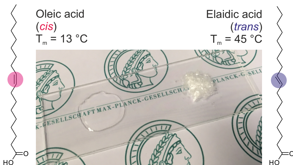
Figure 1.15: Molecular structures and T_m 's of oleic acid (left) and elaidic acid (right). The molecular structures of oleic and elaidic acid only differ in the cis and trans configuration of the double bond. The T_m 's of oleic acid and elaidic acid have a difference of 30 °C. Oleic acids T_m is below and elaidic acids T_m is above room temperature, which explains why oleic acid is liquid and elaidic acid is solid at room temperature.
